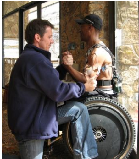
HERL researcher Dany Gagnon attaches surface EMG sensors to athlete and study participant Jake Hipps to compare the amount of muscular effort he needs during wheelchair transfers.
