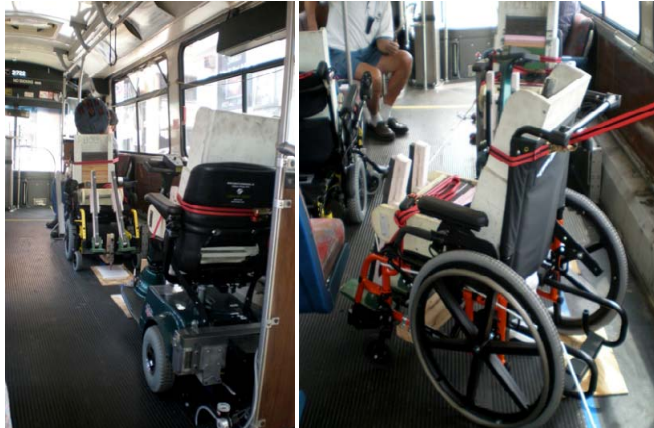
Figure 1 (left): Power wheelchair in the Rear-Facing wheelchair passenger station and Scooter in the Automated Docking System
