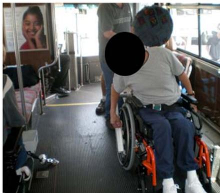
Figure 3: Study participant is evaluating the rear-facing wheelchair passenger station
