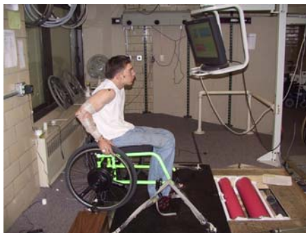
Experimental setup at HERL showing the person and wheelchair secured to the dynamometer and the computer monitor that displays the speed feedback program.
