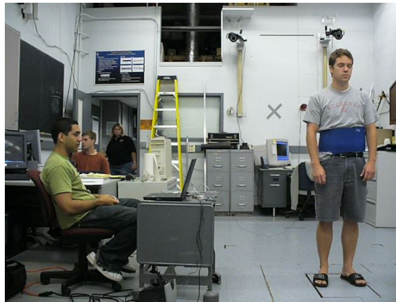
Tomás (L) records data from a sensor attached to the blue waist strap at the Human Movement and Balance Laboratory, while the cameras in the background record motion.
