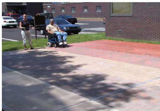
HERL investigators compared vibration levels during manual and power wheelchair propulsion over these six different sidewalk surfaces.
