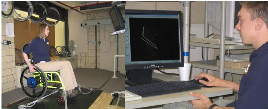
HERL students Jen Mercer (L) and Ian Rice (R) demonstrate the biomechanics lab setup used in this study. As Jen propels, Ian collects her propulsion data from the motion tracking camera system.
