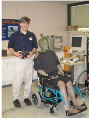
This test dummy was driven in a power wheelchair by remote control over various obstacles in order to observe tips and falls (also pictured: HERL doctoral student Mike Dvorznak)
