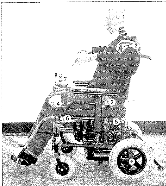
Figure 2. Hybrid III test dummy showing marker locations (1) ear, (2) shoulder, (3) hip, (4) knee, (5) corner of frame (intersection of seat and backrest), (6) front edge of seat, (7) bottom of joystick stem, and (8) top of joystick stem.
